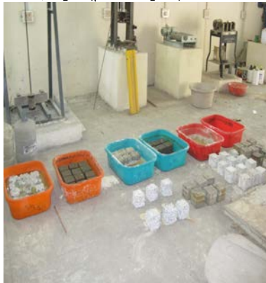
Fig .4 Acid Pond Set up
