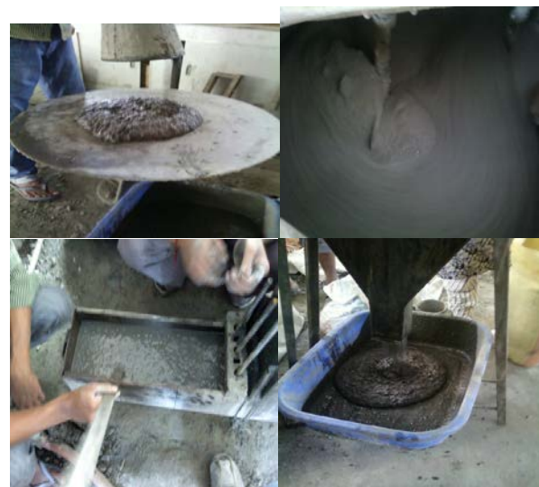
Fig .2 Workability Tests on High Strength Self Compacting Concrete
