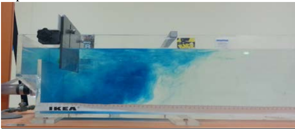
Fig. 2-a Dye pattern at Q=7 L/min, VBS = 11.7 cm, and HBS = 5 cm
