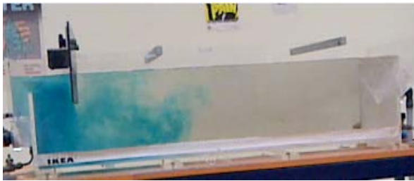
Fig. 4-c: Dye pattern at Q=12 L/min, VBS = 14.1 cm, and HBS = 10 cm
