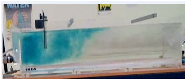
Fig. 5-b : Dye pattern at Q=10 L/min, VBS = 11.7 cm, and HBS = 15 cm
