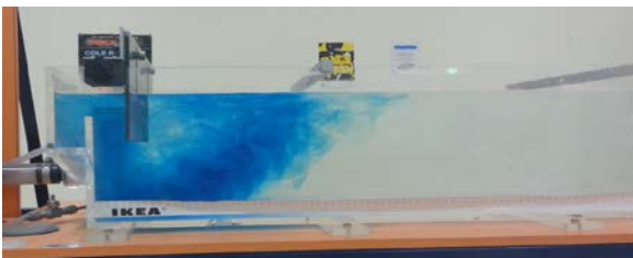
Fig. 2-b Dye pattern at Q=10 L/min, VBS = 11.7 cm, and HBS = 5 cm
