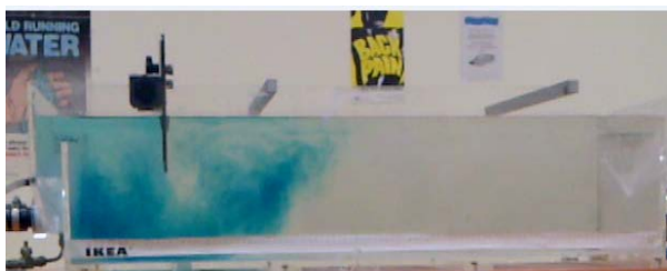
Fig. 5-c: Dye pattern at Q=12 L/min, VBS = 11.7 cm, and HBS = 15 cm
