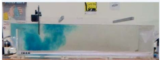
Fig. 5-c: Dye pattern at Q=12 L/min, VBS = 11.7 cm, and HBS = 15 cm
