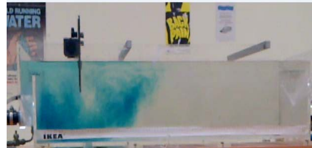
Fig. 6-b: Dye pattern at Q=10 L/min, VBS = 14.1 cm, and HBS = 15 cm
