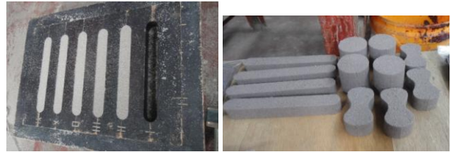
Fig. 1 Moulds and samples for tensile, transverse and compression testing and LOI.
