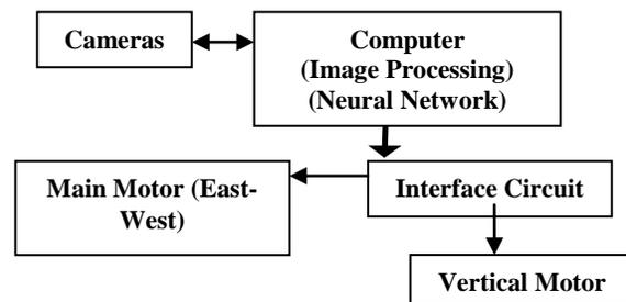
Fig. 1 Experimental setup block diagram
