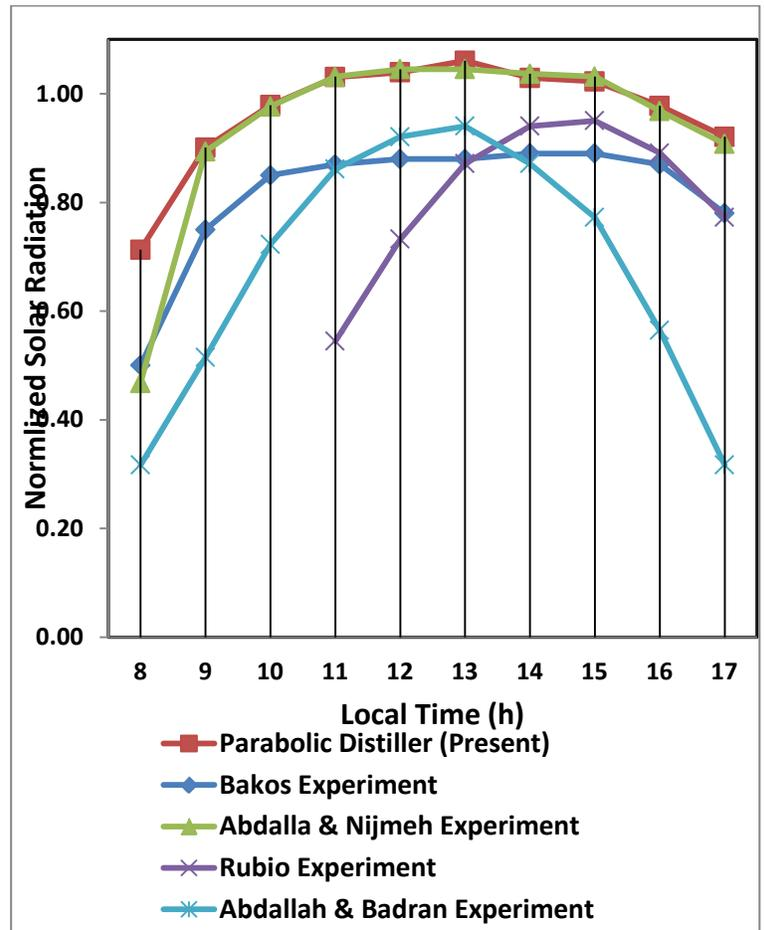
Fig 17. The results of different models of tracking system
