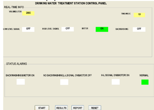
Fig 9: Control Panel GUI
