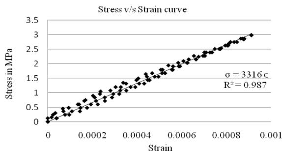
Fig. 1 Stress-strain plot for ACB blocks
