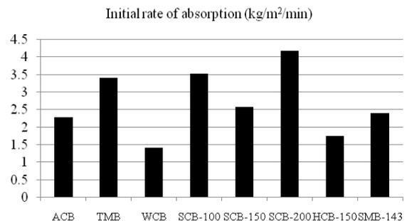
Fig. 2 Comparison of ira values of different types of units
