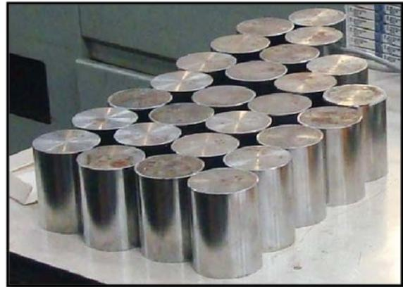
Fig. 2 Samples of chrome coated EN24 steel material
