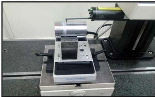
Fig. 3 The probe of the Talysurf Roughness tester
