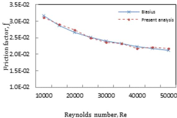
Fig. 1 Comparison of Darcy friction factor by Blasius and computed values for PG/water in turbulent regime.
