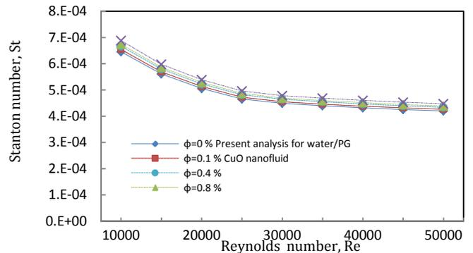
Fig.9. The influence of CuO volume concentration on the Stanton numbers over a range of Reynolds numbers.
