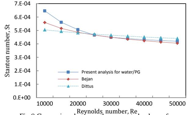
Fig.8 Comparison between the computed values of Stanton numbers and other equation for PG/water
