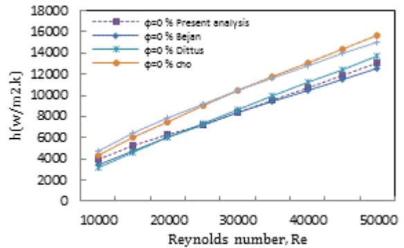
Fig.2. Comparison between the computed values of heat transfer coefficient and other equation for PG/water.
