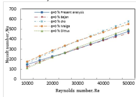
Fig.4. Comparison between the computed values of Nusselt numbers and other equation for PG/water
