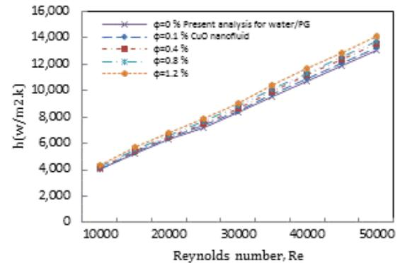
Fig.3. The influence of CuO volume concentration on the heat transfer coefficient over a range of Reynolds number.
