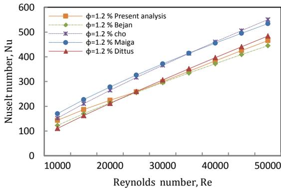
Fig.7 Comparison of Nusselt number for CuO (1.2%) in PG/water with other correlations
