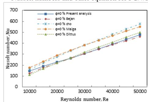
Fig.5 Comparison of Nusselt number for CuO (0.4%) in PG/water with other correlations
