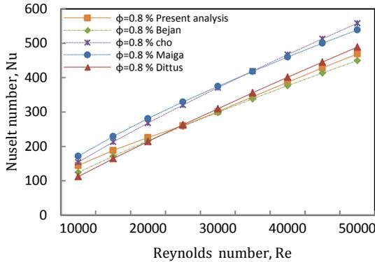
Fig.6 Comparison of Nusselt number for CuO (0.8%) in PG/water with other correlations
