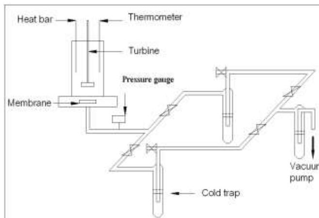
Fig. 1 Schematic diagram of the pervaporation system [8]
