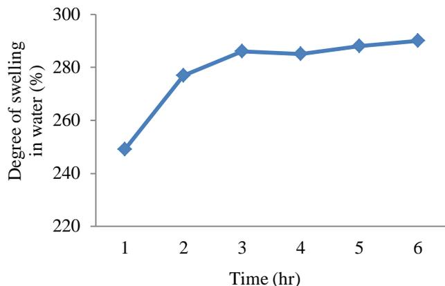
Fig. 2 The degree of swelling in water of the BC-PVA membranes as a function of time
