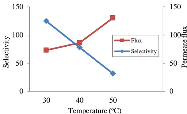
Fig. 4 The effect of temperature on total permeate flux and selectivity
