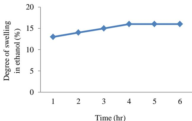
Fig. 3 The degree of swelling in absolute ethanol of the BC-PVA membranes as a function of time
