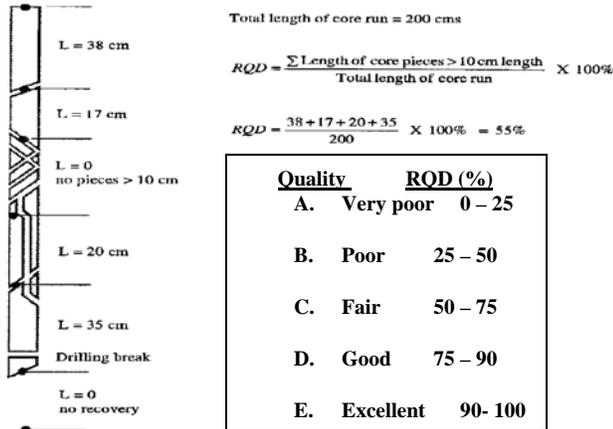
Fig. 2 Procedure of calculating RQD
