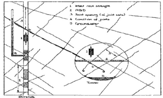
Fig. 1 Showing Parameters of RMR System
