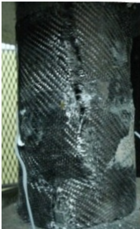
Fig. 3 Typical failure mode of CFRP confined UHPC
