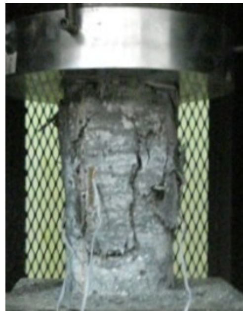
Fig. 2 Typical failure mode of unconfined UHPC
