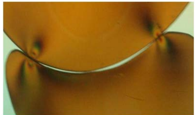
Fig. 5 The pattern of the extrusion punch with load= 5.5 Kg
