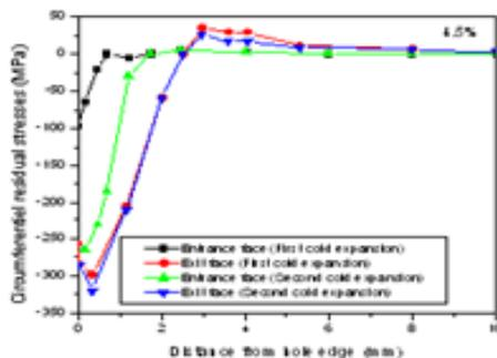
Fig. 3 Residual stresses distribution for the first and the second pass of cold expansion process
