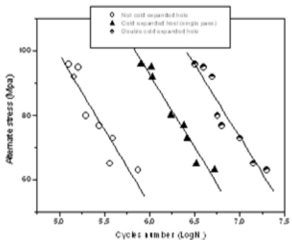
Fig. 4 Wöhler curves for the three batches of specimens
