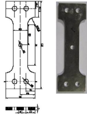
Fig. 1 Specimens geometry and dimension (mm)
