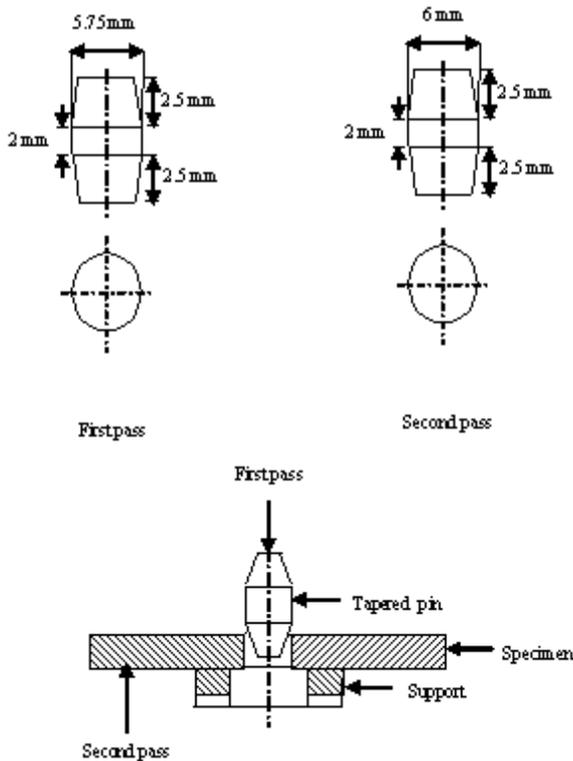
Fig. 2 Double cold expansion process using tapered pins
