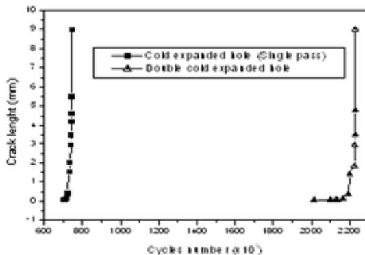
Fig. 6 Comparison of cracks growth (Single pass and double pass)
