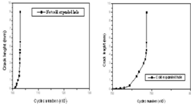
Fig. 5 Comparison of cracks growth (Not expanded hole and cold expanded hole – Single pass)
