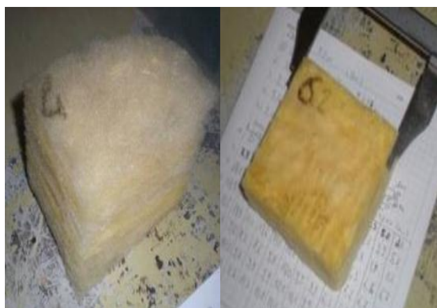
Fig. 5 Visual observation of a new sample (N3, on the left) and an old aged sample (C3, on the right)
