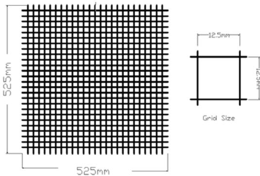
Fig. 2 Polymeric reinforcement details
