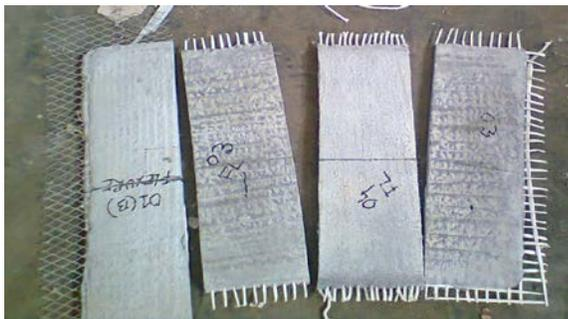
Fig. 5 Crack in Tested Specimens
