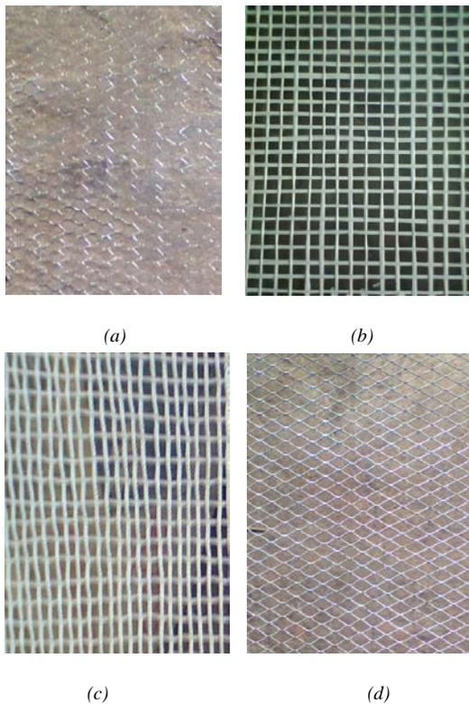
Fig. 1 Types of mesh. (a) Hexagonal iron mesh, (b) Woven PP, (c) Woven Nylon 66 (d) Expanded Metal mesh
