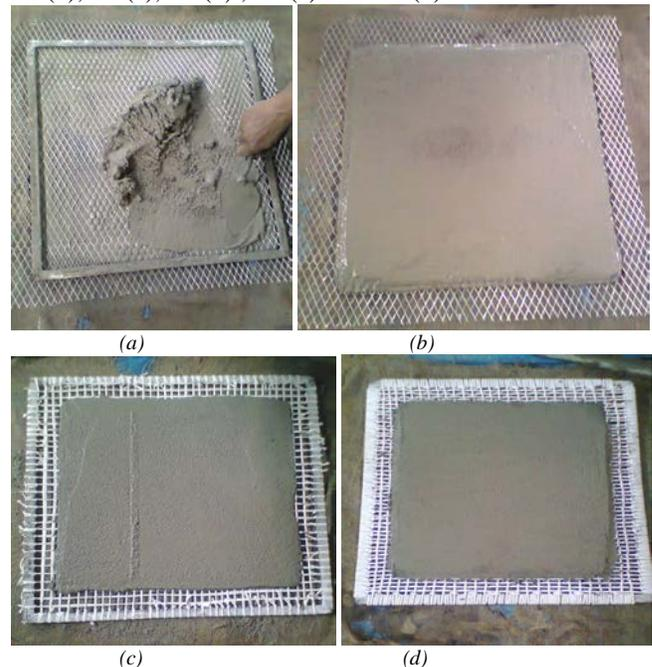
Fig. 3 Test specimens (a) preparation of ferrocement slabs (b) specimen with expanded metal mesh, (c) PP mesh, (d) nylon 66 mesh.
