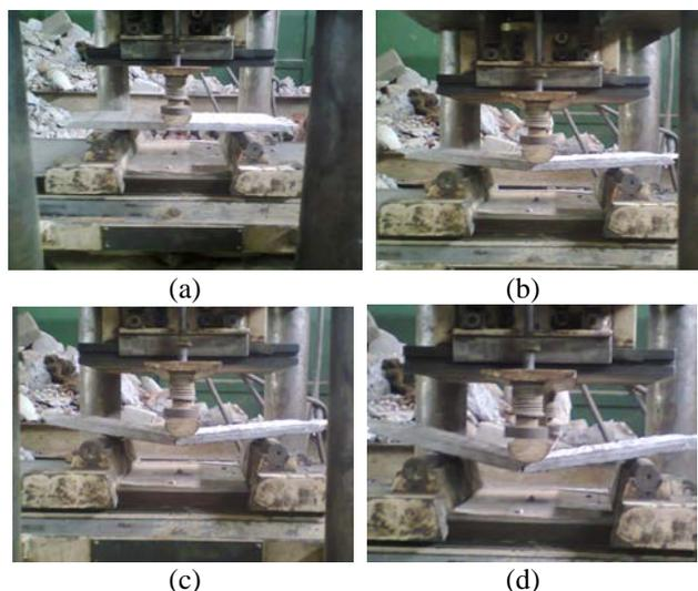
Fig. 4 Flexural test method (one point load) from initial to ultimate load situation
