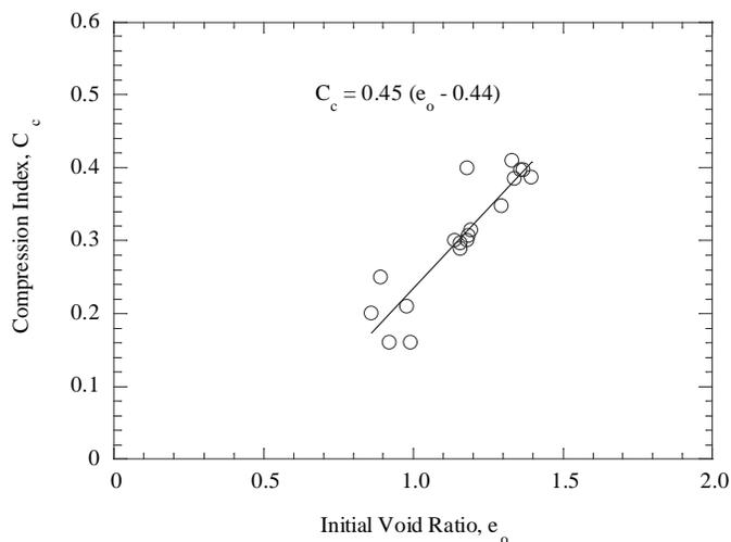
Fig. 3 Compression index versus initial void ratio of coastal soil
