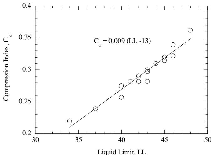
Fig. 5 Compression index versus liquid limit
