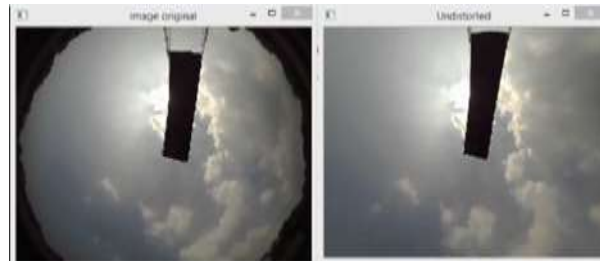
Fig. 5.Sky image before and after calibration
