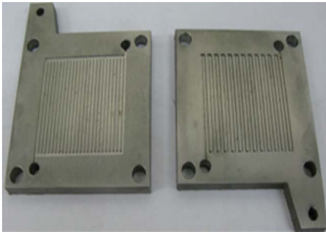
Fig .1 Spiral and Parallel Channels (Bipolar Stainless Steel)
