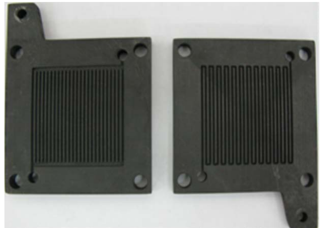
Fig. 3 parallel and spiral graphite channels.
